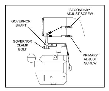
Figure 10. Engine Governor Adjustment Single Cylinder Engines
